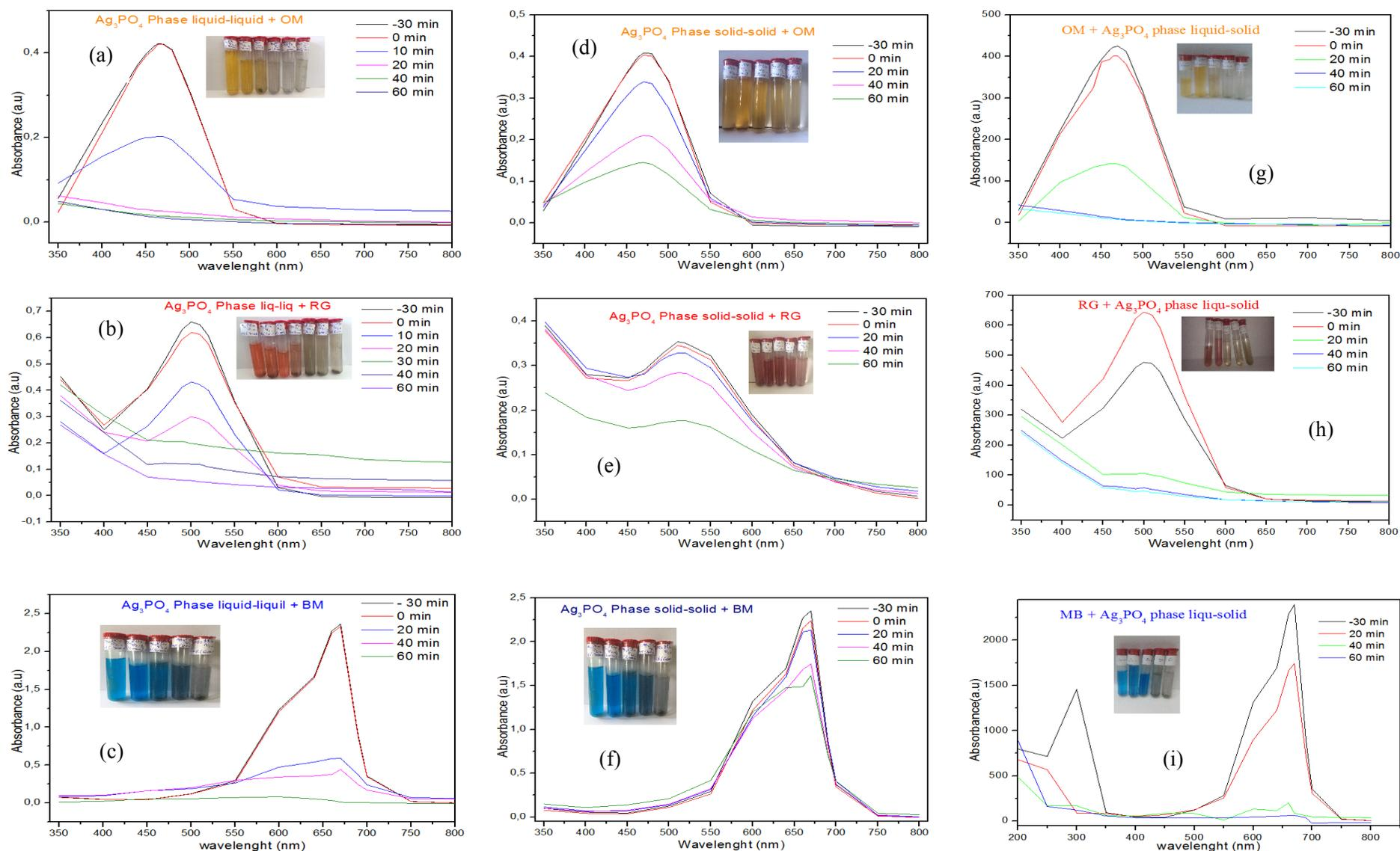
**Figure 3:** UV-visible absorption of three dyes (OM, RG, BM) photocatalysed by (a-c)  $\text{Ag}_3\text{PO}_4$  L-L, (d-f)  $\text{Ag}_3\text{PO}_4$  S-S and (g-i)  $\text{Ag}_3\text{PO}_4$  L-S
