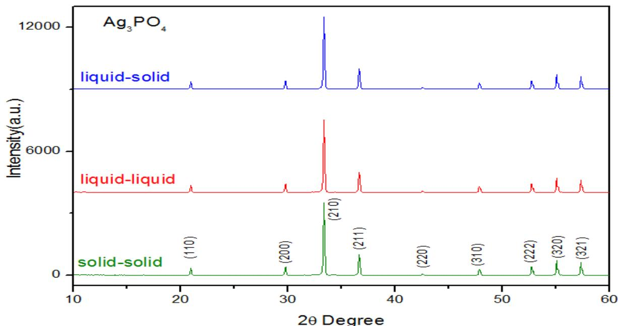
**Figure 1:** XRD patterns of the  $\text{Ag}_3\text{PO}_4$  photocatalysts prepared with different methods
