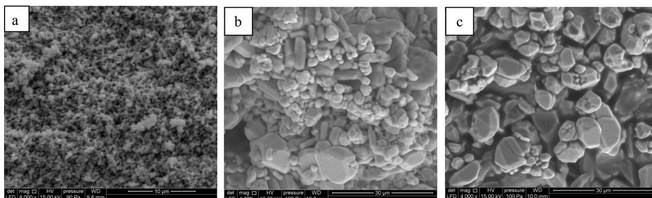
**Figure 2 :** SEM images of the samples prepared with different methods: (a)  $\text{Ag}_3\text{PO}_4$ L-L, (b)  $\text{Ag}_3\text{PO}_4$ L-S and (c)  $\text{Ag}_3\text{PO}_4$ S-S
