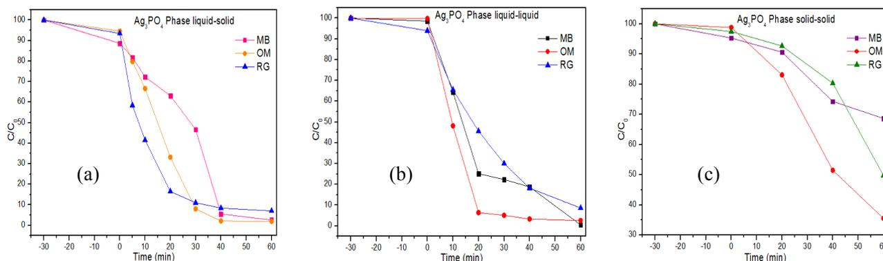
**Figure 4:** Photocatalytic degradation of OM, MB and CR by the as-prepared photocatalysts (a)  $\text{Ag}_3\text{PO}_4$  L-S (b)  $\text{Ag}_3\text{PO}_4$  L-L and (c)  $\text{Ag}_3\text{PO}_4$  S-S under visible-light irradiation.
